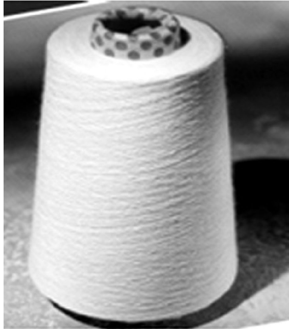
CONE 90–150 mm height diameter of nearly 300 mm cone angle from 4^{\circ}20' to 11^{\circ} 2–3 kg of yarn 50–100 km length
