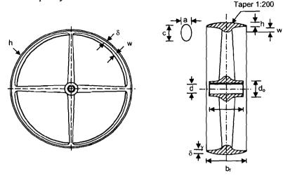
Figure 9.5 : A Pulley with Arms Connecting Hum and Rim
