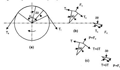
(a) A Belt Round a Pulley. Pulley Rotates in Direction of  $T_t$
