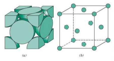
Figure 3.1 For the facecentered cubic crystal structure, (a) a hardsphere unit cell representation, (b) a reduced-sphere unit cell, and (c) an aggregate of many atoms. [Figure (c) adapted from W. G. Moffatt, G. W. Pearsall, and J. Wulff, The Structure and Properties of Materials, Vol. I, Structure, p. 51. Copyright @ 1964 by John Wiley & Sons, New York. Reprinted by permission of John Wiley & Sons, Inc.]
