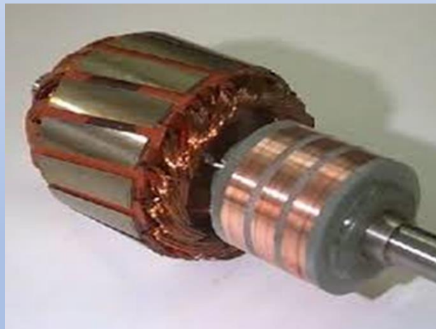
Slip Rings mounted on Shafts Three rings for 3 phase M/c
