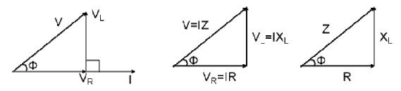
The impedance triangle is right angled triangle with R and  $X_L$  as two sides and impedance as the hypotenuse. The angle between the base and hypotenuse is  $\Phi$ . The impedance triangle enables us to calculate the following things.
