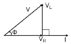
The current I is taken as the reference phasor. The voltage  $V_R$  is in phase with I and the voltage  $V_L$  leads the current by 90°. The resultant voltage V can be drawn as shown in the figure. From the phasor diagram we observe that the voltage leads the current by an angle  $\Phi$  or in other words the current lags behind the voltage by an angle  $\Phi$ .
