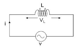
Consider an AC circuit with a pure inductance L as shown in the figure. The alternating voltage v is given by  $v = V_m \sin \omega t$  \_\_\_\_\_(1)
