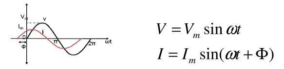
From the phasor diagram, the expressions for the resultant voltage V and the angle  $\Phi$  can be derived as follows.
