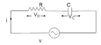
Consider an AC circuit with a resistance R and a capacitance C connected in series as shown in the figure. The alternating voltage v is given by
