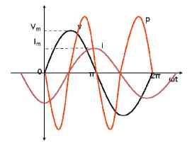
As seen from the power waveform, the instantaneous power is alternately positive and negative. When the power is positive, the power flows from the source to the inductor and when the power in negative, the power flows from the inductor to the source. The positive power is equal to the negative power and hence the average power in the circuit is equal to zero. The power just flows between the source and the inductor, but the inductor does not consume any power.
