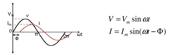
From the phasor diagram, the expressions for the resultant voltage V and the angle  $\Phi$  can be derived as follows.
