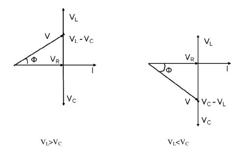
From the phasor diagram we observe that when  $V_L > V_C$ , the voltage leads the current by an angle  $\Phi$  or in other words the current lags behind the voltage by an angle  $\Phi$ . When  $V_L < V_C$ , the voltage lags behind the current by an angle  $\Phi$  or in other words the current leads the voltage by an angle  $\Phi$ .
