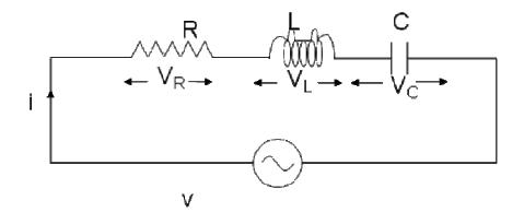
Consider an AC circuit with a resistance R, an inductance L and a capacitance C connected in series as shown in the figure. The alternating voltage v is given by
