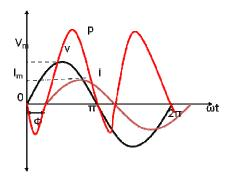
As seen from the power waveform, the instantaneous power is alternately positive and negative. When the power is positive, the power flows from the source to the load and when the power in negative, the power flows from the load to the source. The positive power is not equal to the negative power and hence the average power in the circuit is not equal to zero.
