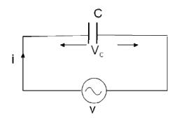
Consider an AC circuit with a pure capacitance C as shown in the figure. The alternating voltage v is
