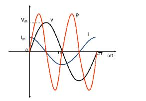
As seen from the power waveform, the instantaneous power is alternately positive and negative. When the power is positive, the power flows from the source to the capacitor and when the power in negative, the power flows from the capacitor to the source. The positive power is equal to the negative power and hence the average power in the circuit is equal to zero. The power just flows between the source and the capacitor, but the capacitor does not consume any power.
