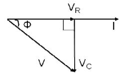
The current I is taken as the reference phasor. The voltage  $V_R$  is in phase with I and the voltage  $V_C$  lags behind the current by 90°. The resultant voltage V can be drawn as shown in the figure. From the phasor diagram we observe that the voltage lags behind the current by an angle  $\Phi$  or in other words the current leads the voltage by an angle  $\Phi$ .
