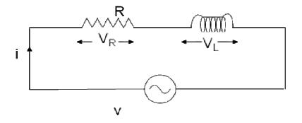
Consider an AC circuit with a resistance R and an inductance L connected in series as shown in the figure. The alternating voltage v is given by
