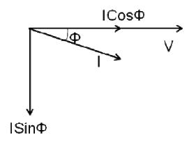
From the phasor diagram of an RL series circuit, the current can be divided into two components. One component along the voltage  $Icos\Phi$ , that is called as the active component of current and another component perpendicular to the voltage  $Isin\Phi$  that is called as the reactive component of current.
